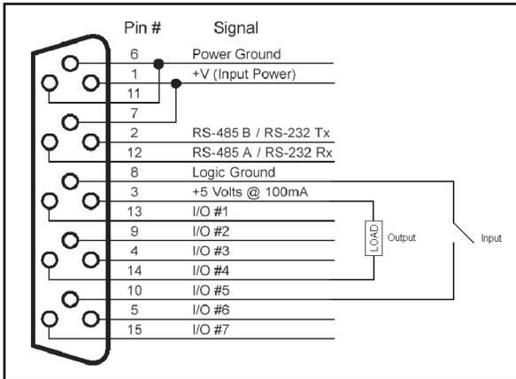
These signals provide power, communications and 3.3v IO signals (digital and analog).
