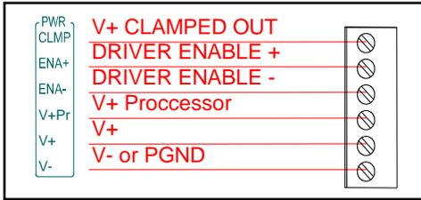
The two main items are V+ & V-, normally from the main power supply. V+Pr is a separate power input to keep the processor alive for certain applications. ENA+ and ENA- are inputs to an optically isolated drive enable. If Driver Enable is not needed, jumper ENA+ to CLMP and ENA- to V-. CLMP is a fused 150 mA output. CLMP = V+ minus 0.3V.
