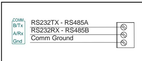
Standard RS-232/RS-485 connections broken out to terminals for easy wiring.
