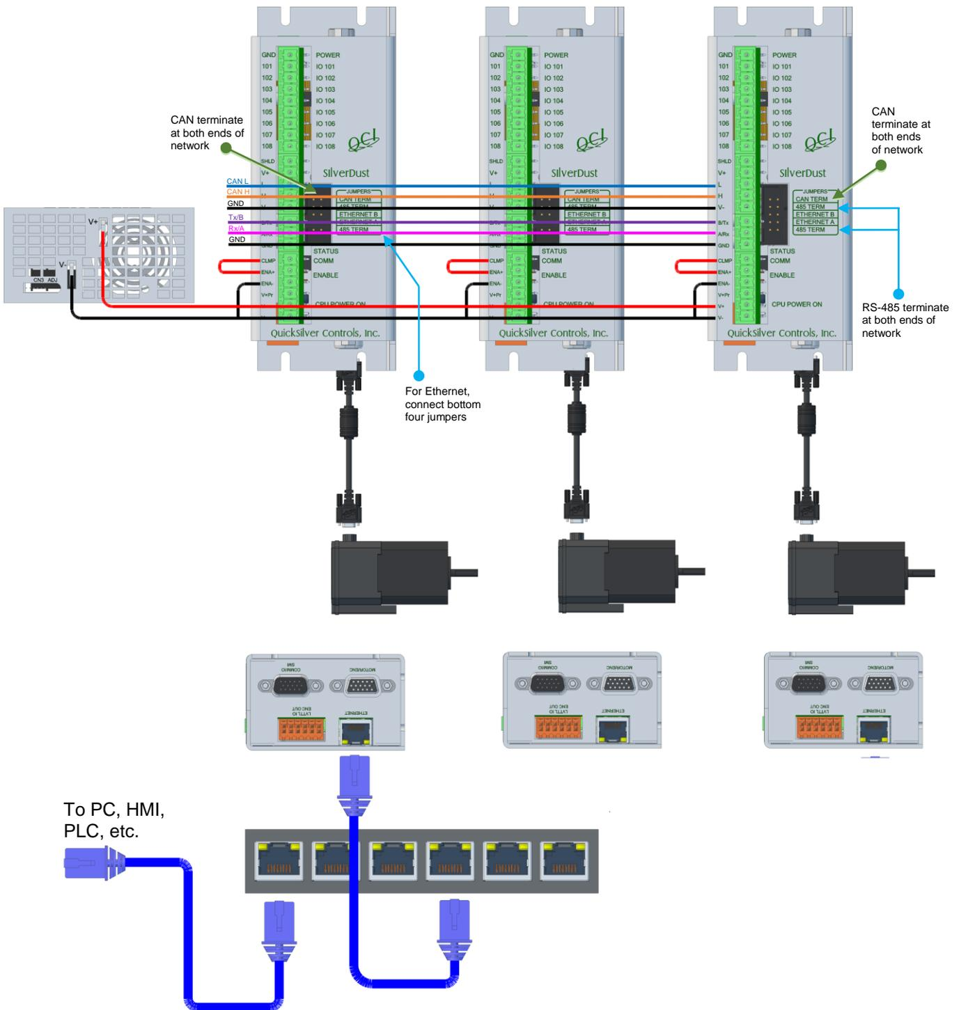
This configuration shows a three-axis system, consisting of one QCI-D2-IGM-E with two QCI-D2-IGM controllers. The E-485 Bridge provides a bridge between Ethernet and RS-485, providing communications to all 485 connected controllers. One Ethernet connection using one IP address communicates with a whole network of QuickSilver servo controllers.
