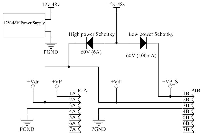
Power is isolated from DB15HD SIP port, pins 1&7 with this configuration.
