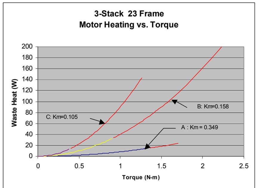
The lower curve is Step motor, A, the middle curve is BLDC motor B, and the upper curve is BLDC motor C. The red portions of each curve represent the motor as it is operated beyond continuous torque rating, but within the peak torque performance rating.
